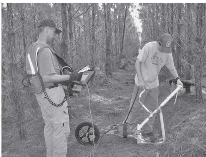
FIGURE 12.50 SIR 2000 ground-penetrating radar (GPR) system connected to a 1500 MHz antenna mounted on a skateboard deck equipped with a survey wheel encoder.
